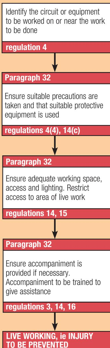
85 The procedures associated with live working are illustrated in Figure 5. While it is not always possible to follow rigidly a set procedure to cover all situations, you should follow the management principles described in this guidance and the safe system of work criteria set out in paragraphs 25–32.
